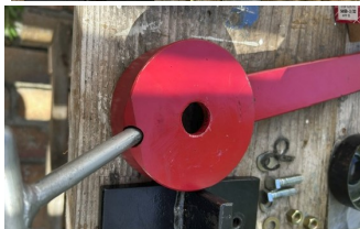
Mount shock base to holding fixture, before clamping in sturdy vice.
